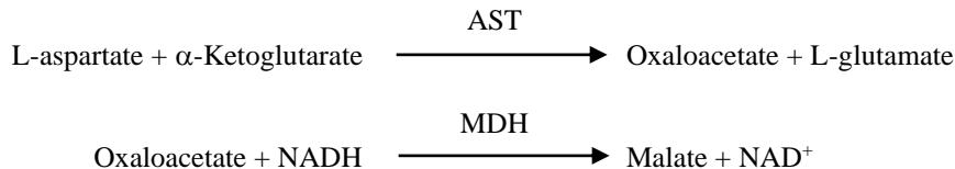
The rate of absorbance change to 340/405 nm caused by the conversion of NADH to NAD<sup>+</sup> is directly proportional to the amount of AST present in the sample.
