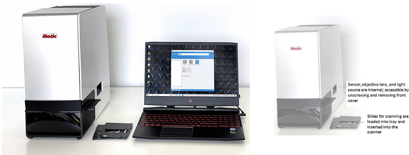
Figure 2. The EasyScan One scanner (Motic) has dimensions of 20 \times 40 \times 42 cm, and must be connected physically (wired) to a control laptop with a graphic processing unit capable of handling images.
