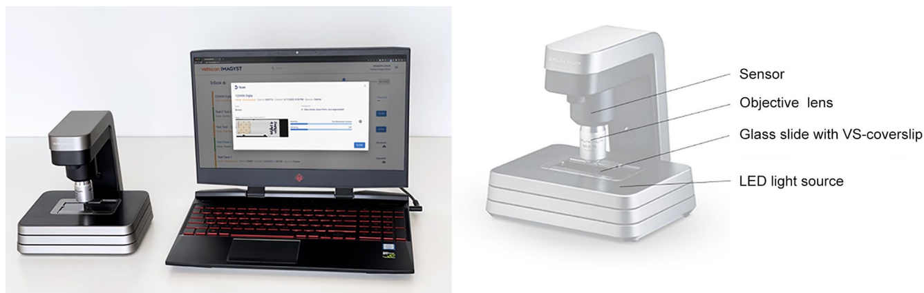
Figure 1. The Ocus 40 scanner (Grundium) has dimensions of 18 \times 18 \times 19 cm, and contains an integrated graphic processing unit, allowing a user interface with a basic internet-connected device (laptop shown for scale).
